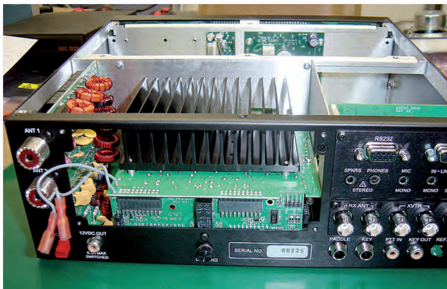
And in goes the r.f. power amplifier module with its finned heatsink. The two fans on the back panel blow air across the fins.
